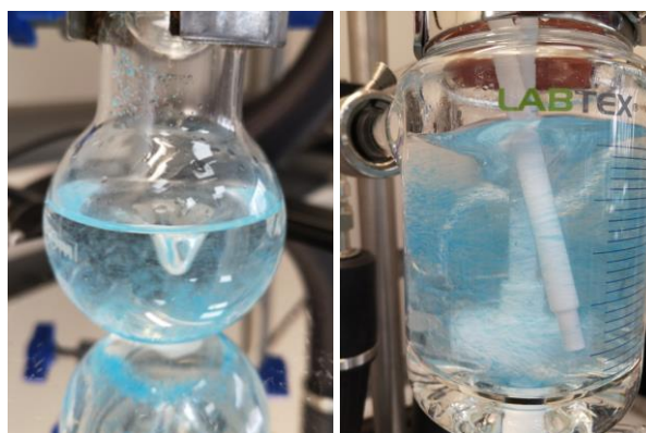
Figure 1: Comparison of stirring between magnetic stirrer ( left ) and mechanical stirrer with impeller ( right )
